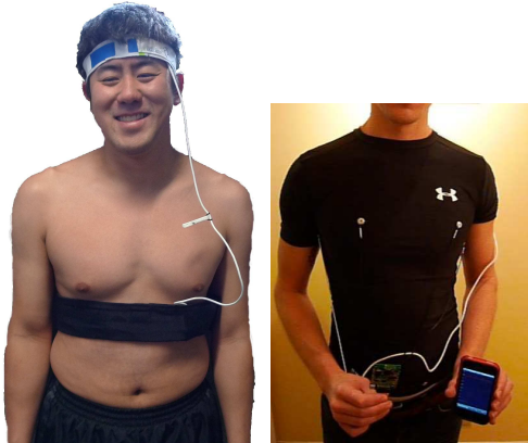
Figure 2: Left: Chest belt containing Tricorder and electrodes, reflective forehead pulse-ox sensor. Right: Compression shirt with conductive fabric on the inside, data visualization on iPhone.
